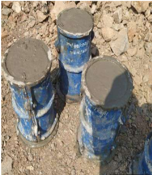
Figure 5: Casting of cylinders for split tensile test
